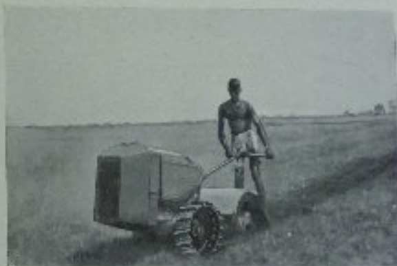
Fig. 3—The Simar Rototiller 10 is a compact machine which is easily converted into a machine between closely planted crops.
